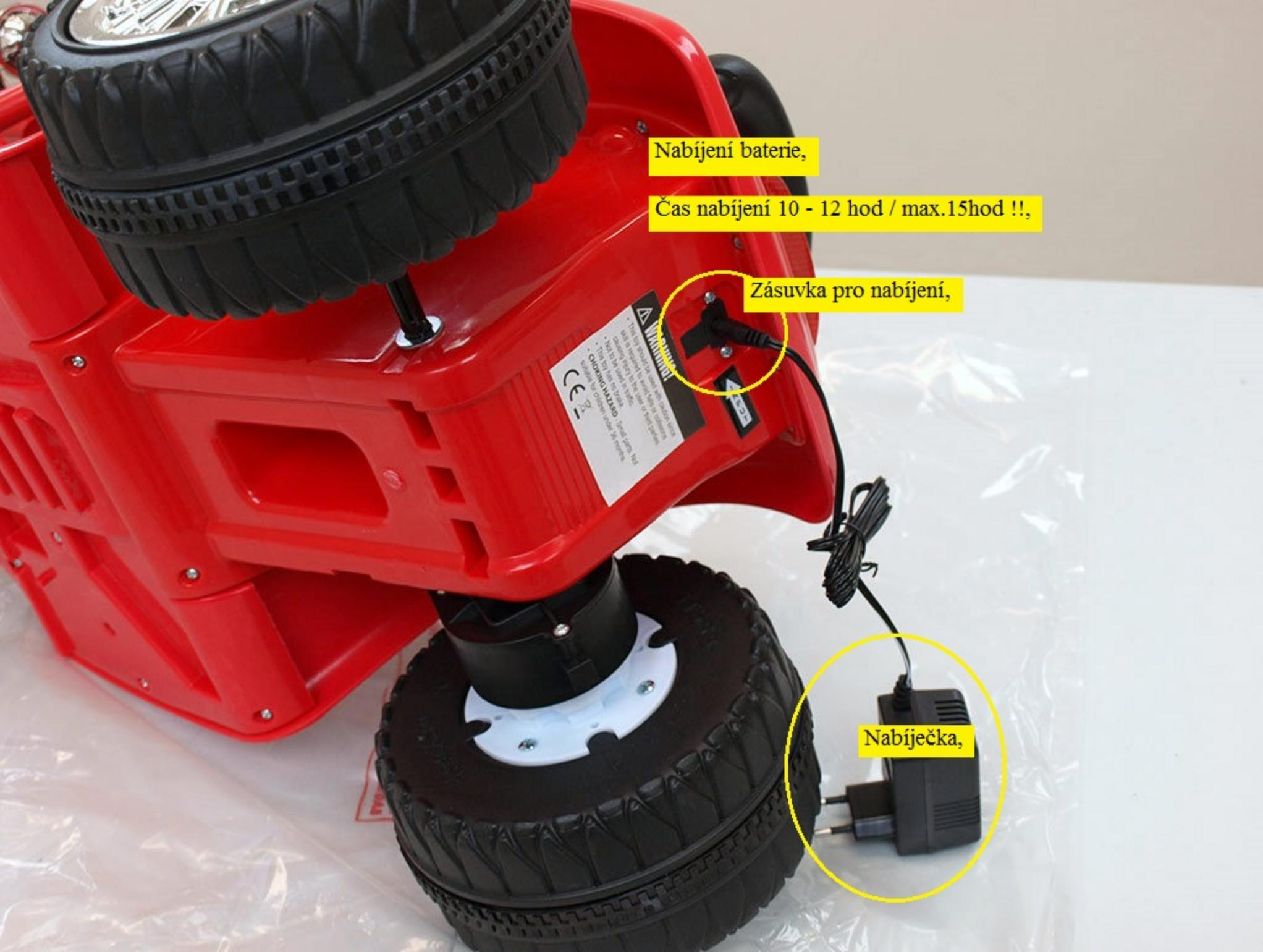
A red toy car is shown from a rear-quarter perspective. The car has two large black tires with a tread pattern. A red battery pack is mounted on the back. A black charging cable is plugged into a port on the battery pack. A black power adapter is connected to the other end of the cable. The car is resting on a white plastic surface.
